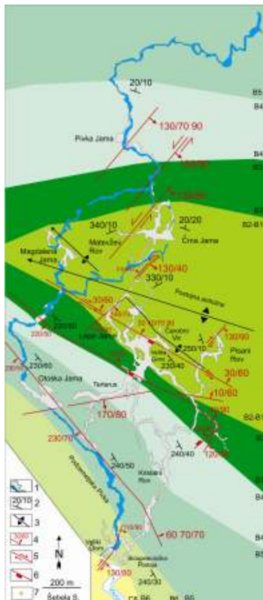
Fig 1. Geology of Postojna Cave System. 1-cave passage with underground River Pivka, 2-strike and dip direction of bedding plane, 3-anticline, 4-strike and dip direction of fault, 5-dextral horizontal movement, 6-vertical movement, 7-subsidence of SW block.
